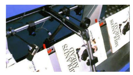
The reject collection tray is accessible and visible from both sides of the machine and has a large pile height capacity.
