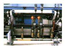
The Pacesetter 5P705 stitcher is of the reciprocating shuttle design. A heavy duty cast iron lower base construction with modular upper sections offers improved durability and long term, high speed reliability. Shuttle stroke may be matched to the chain pitch setting and is changed by a switch on the control panel and a simple mechanical adjustment. Significant noise reduction is achieved through the use of a polyurethane dampened shuttle gripper system and improved machine guarding.
