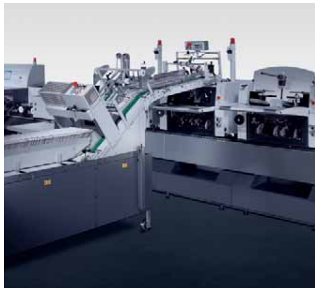
Continual loading with a stream feeder.
