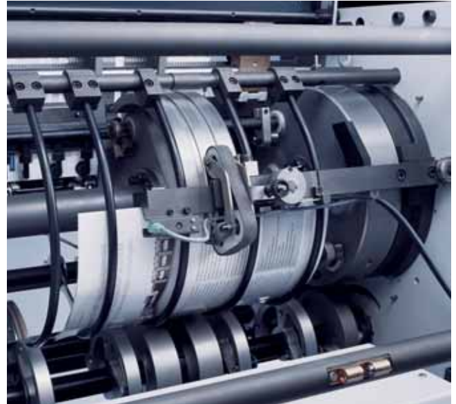
A patented register stop belt prevents damage to sheets in the feeders.
