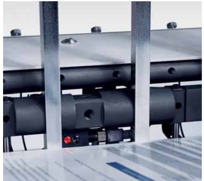
Remaining pile monitoring at each feeder prevents its magazine from running out.
