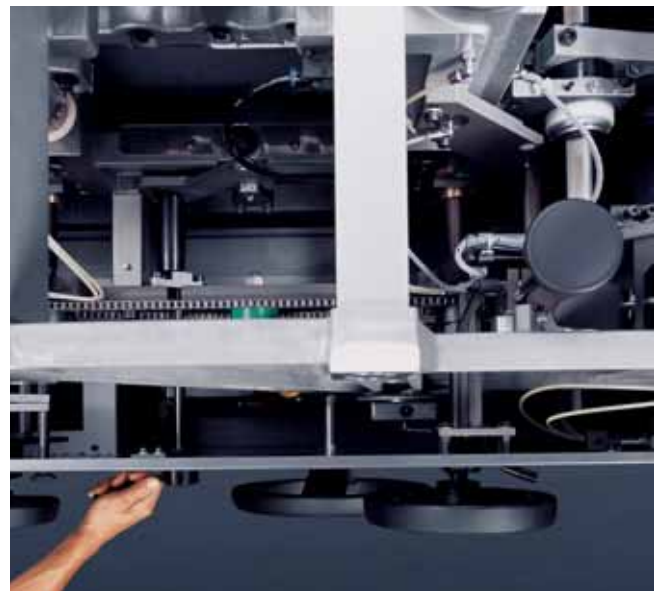
The two bed knife blocks are clamped on the operator side.
