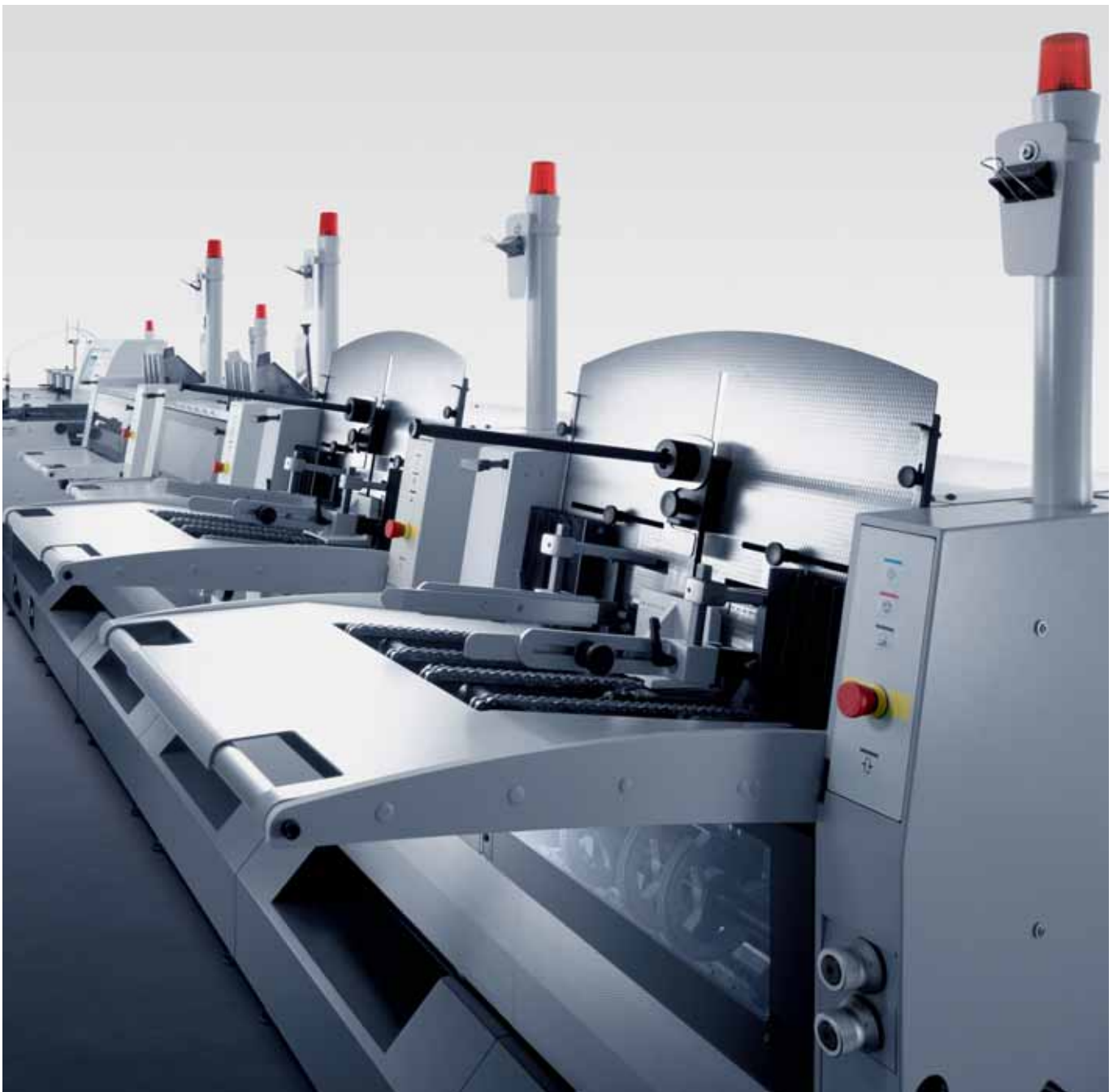
The vertical feeders reduce pressure on the signatures.
