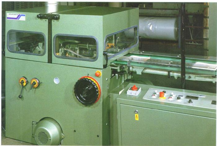
The 3-knife trimmer is an important component of an efficient production line. Saddle stitcher and 3-knife Accurate a trimmer should be carefully matched to assure consistent output and product quality.
