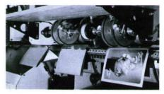
Once opened, signature drops smoothly on bayonet. Pusher fingers move opened signature off bayonet and onto crowned conveyor chain in perfect register. Exceptionally short signature drop assures precise positioning.
