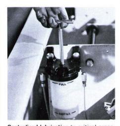
Centralized lubrication to critical areas, supplemented by easily-accessible grease fittings, keep maintenance time to a minimum.
