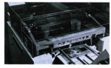
Register Belt controls the book throughout the trimming operation. Belt stops when book is being trimmed so there is no marking from belt slippage.
