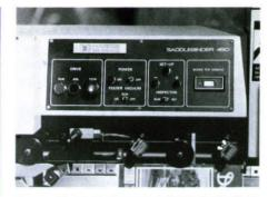
**Control Zone design** centralizes controls at the stitcher and every second station for operator convenience.
