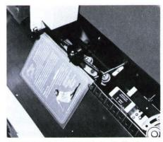
Shuttle guide consists of sturdy, firmly supported hardened shafts that let shuttle convey signatures smoothly at all operating speeds.
