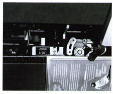
5. **Set inspector** by flicking "set" switch and jogging machine until "set-up" light comes on. Unlock inspector wheel, place sample book under it, move detector collar into position and lock. Release detector collar and you're set to detect both "unders" and "overs."
