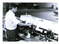
Operator efficiency is increased by simple, compact, easy-to-operate design. Pockets are 18" (457 mm) center to center and only 4 feet (1219 mm) high to reduce the "reach" required for loading. One-side loading/operating feature permits space-saving positioning against the wall.
