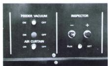
"Air Curtain", standard equipment, applies air pressure to either side of signature to hold it firmly on conveyor chain and prevent flare-out at high speeds. Separate air pump is mounted on main frame.
