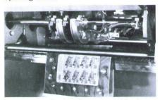
Once opened, signature smoothly drops on bayonet above crowned conveyor chain. Pusher fingers move opened signature off bayonet and onto conveyor chain in perfect register. Exceptionally short signature drop assures precise positioning. Conveyor chain can be raised if ever required.
