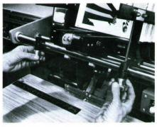
6. Set hoppers. Loosen two knobs and move guides to signature size. Tighten knobs. Untrimmed signatures from  $3\frac{1}{2}$  x  $5\frac{3}{4}$ " to  $12\frac{1}{2}$  x  $20\frac{3}{4}$ " (89 x 146 to 317 x 527 mm) can be handled. Reply cards with  $1\frac{1}{2}$ " (38 mm) hanger can be fed at any station.
