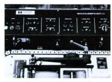
Control Zone design that centralizes controls at stitcher and every second station, makes the unit easier to operate than ever.
