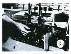
4. **Set stitcher heads.** Loosen lock levers and move heads into desired position. Align the clinchers. Dial the correct wire feed for book thickness.
