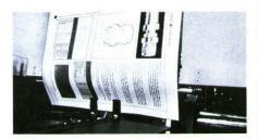
Signature is effortlessly separated by telescoping suckers and conveyed by grippers on the transfer wheel. Grippers positively place signature in precise position against register stops in the transfer cradle.
