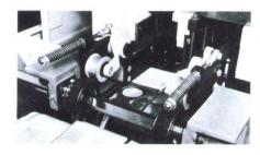
The fourth and fifth knife attachment is self-centering and can be installed in just 15-20 minutes. There is no need to install supplementary chains to convey center trimmed books out of the trimming area.
