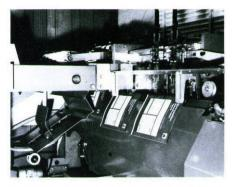
3. Center book for trimmer entry. Release lever to declutch conveyor chain. Move chain and conveyor finger to contact book. Lock lever.
