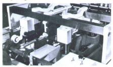
**Trimmer uses 2**½" (57 mm) square knife bar supports for greater strength. Open design provides easy chip removal.
