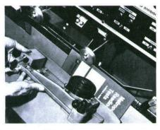
5. Set pack inspector. Flick "set" switch. Jog machine until keyway on the inspector wheel is in the up position. Unlock wheel, place sample book under it, move detector collar into position and lock the wheel into position. Release detector collar. Inspector is adjustable and detects both "under" and "over."
