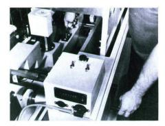
1. Set trimmer. Release quick-acting hand clamps and move knives to position for head and foot dimension. Loosen lever on register stops and move to face cut dimension. Loosen clamp and slide sideguides to signature dimension for precise entry into trimming area.
