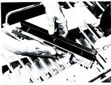
Dies are two matched pieces for easy installation and are self-aligning to speed set-up.
