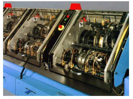
The operator has an open view and access to all mechanisms on the signature flow path, so set-up is quick, easy and tool-less.
