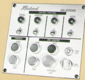
Built-in central control panel permits pushbutton operation of feeding, stitching and trimming functions for easy set-up and operation. Contains built-in timing light so machines can be timed to provide maximum production. Individual functions—feeding and stitching, trimming and stitcher heads—can be controlled independently or in combination for set-up. Panel lifts up for easy access to internal electrical functions.
