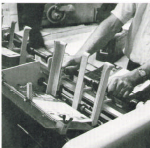
Set-up of the Saddle-Matic 66 is the simplest yet. Here the pile guides on the pocket are being adjusted with the large wing-nuts. Two adjustments set-up the pocket for lap signature . . . time: 20 seconds per pocket; for signatures without lap, about 70 seconds total.
