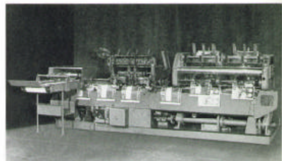
The basic unit consists of (right to left) two feeder pockets, caliper and stitcher all mounted on the same base. Additional pockets (units of two), hand-feed stations and/or automatic 3-knife trimmer can be added at any time.
