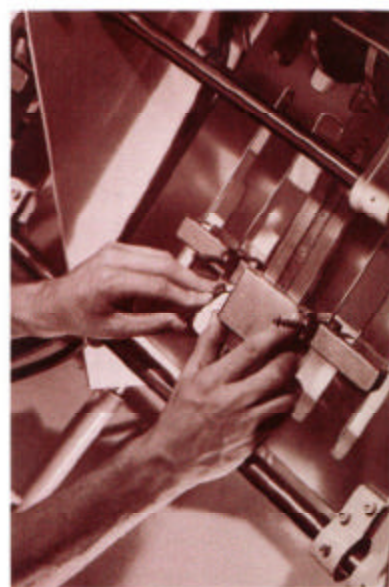
Adjustment of the backbone register gauge in the pocket is done on a direct reading scale. The gauge has a patented deflector that gives the signature ample room coming into the gauge, then compresses to guarantee perfect register, prior to lap grippers closing.
